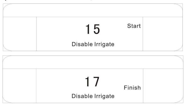
(5) During forbidden irrigation time, manual open the magnetic valve, the magnetic valve will keep open, the words "Disable Irrigate" will disappear from the LCD. Manual close valve, will back to auto status.
