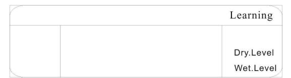
Use the up/down key to cause an icon, which represents an item to set up, to flash, and then select the item by pushing the, "ENT", Enter key to setup (Details see following). Push the exit key, "EXT" to exit. If 20 seconds elapses before a key is pushed the controller will exit from the set up mode, pushing any key while an icon is flashing time will begin a 20 second period to allow data entry again.
